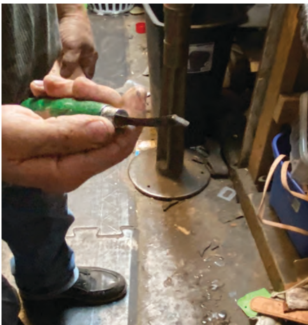
A Lip Knife is used in shoe repair to cut excess leather.
