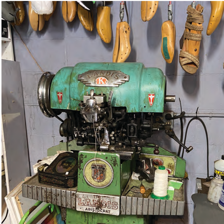
Shoe Stitcher. The most important machine in the shop, stitches sole edging all the way around the shoe by inserting the shoe upside down.
