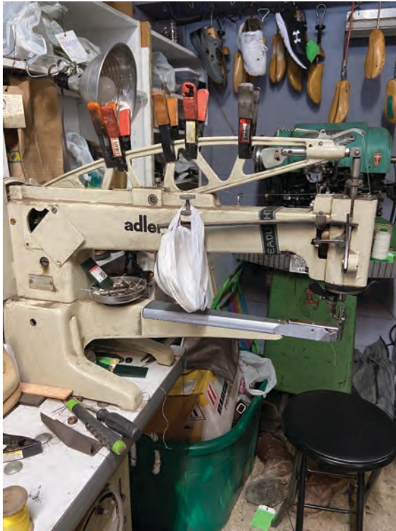
Patcher. This machine can sew patch onto thick leather.
