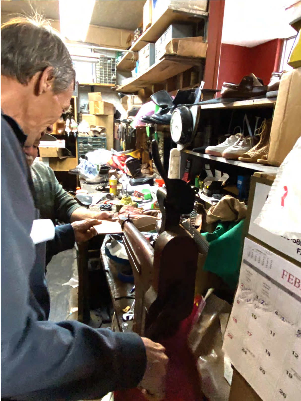
Kevin is using a “5 in 1” machine to cut out a leather insole.
