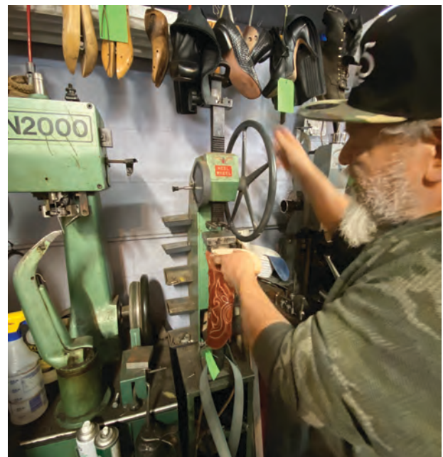
Heel Wheel. This machine presses nails up into the boot heel. A wire heel nailer pushes wire into a rubber heel so you don't have to use nails.
